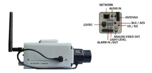
This Wireless High Resolution H.264 IP camera has a built-in web server that can be used to view and administrate the camera. In addition, the camera comes with our exclusive 16 channel VR Series Virtual DVR Client software. The Virtual Client will allow you to view and record the camera over the network, and to combine the camera with other VR Series components to create a complete enterprise-wide security solution.
